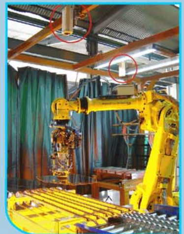
Palletising of glasses through Machine Vision
